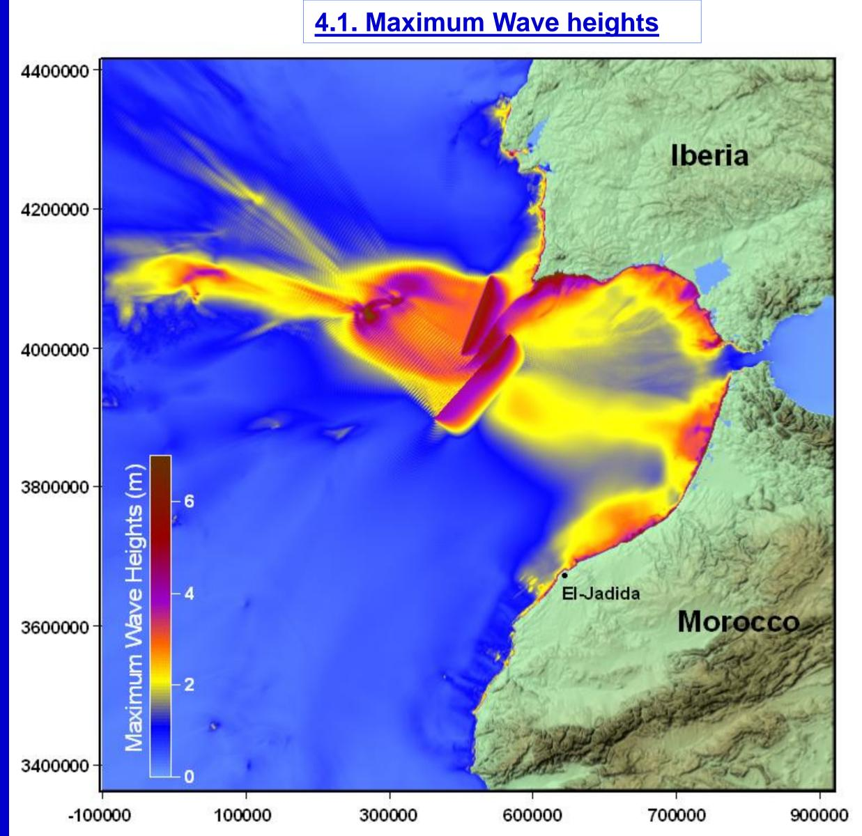
■ Figure. 4. Computed Tsunami Maximum Wave heights distribution in the Gulf of Cadiz area due to the occurrence of the MPF/HSF submarine earthquake scenario
