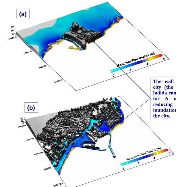
The wall of the Portuguese city (the old Medina) of El Jadida can act as a protection for 6 m tsunami wave, reducing the tsunami inundation risk in this part of the city.
