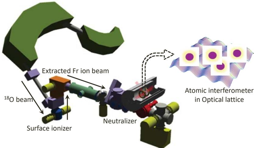
**FIGURE 1.** The overview of the EDM apparatus. The primary beam of  $^{18}\text{O}$  is injected to the  $^{197}\text{Au}$  target installed in the surface ionizer. The Fr produced in the target is extracted as ion, and transported to the neutralizer, and moved to the MOT and OL to measure the EDM with atomic interferometer.
