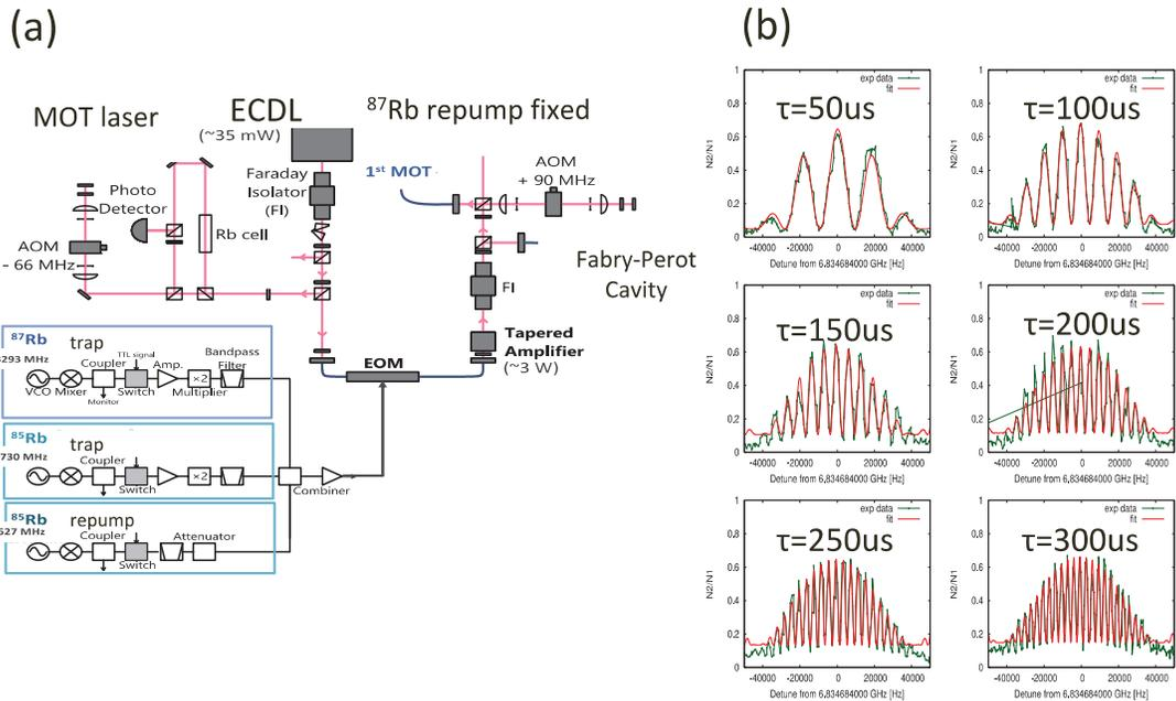
**FIGURE 4.** The left figure shows the laser optics for the MOT to trap the dual species atoms such as  $^{85}\text{Rb}$  and  $^{87}\text{Rb}$  with an ECDL. The right plots show the interference pattern of Ramsay resonance with the change of interaction time from 50  $\mu$ s to 300  $\mu$ s. The peak width corresponds to the resolution of the EDM measurement, and to achieve the sensitivity  $10^{-30}$  ecm, interaction time of 1~10 s will be required.
