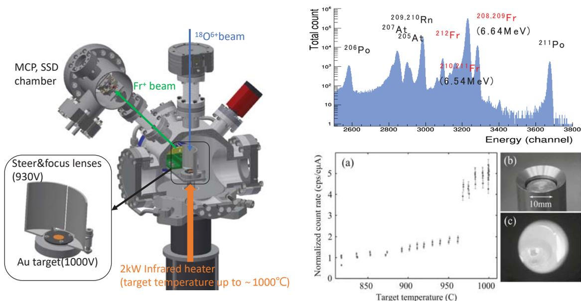
**FIGURE 2.** The structure of the surface ionizer is shown in the left figure. The right upper plot shows the spectrum of produced RIs measured by SSD. The right lower plot shows the temperature dependence of the produced Fr yield. Above the melting point of  $^{197}\text{Au}$  ( $1064^\circ\text{C}$ ), the production yield is drastically increased.
