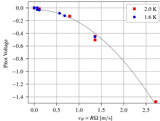
**Figure 13.** Mean voltage of the miniature Pitot sensor for several mean azimuthal velocities and temperatures in He II (1.6 K and 2.0 K). The dashed line is a quadratic fit.
