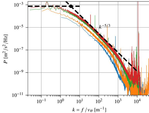
**Figure 18.** Velocity power spectra obtained in He I (2.3 K) in *co-rotation* with the hot-wire as a function of the wave number  $k$ . From bottom to top:  $\Omega = 0.19 \text{ rad/s}$ ,  $\Omega = 0.50 \text{ rad/s}$ ,  $\Omega = 2.20 \text{ rad/s}$ ,  $\Omega = 3.77 \text{ rad/s}$ . The black dot is  $k_0 = 3.48 \text{ m}^{-1}$  at the intersection of the  $k^{-5/3}$  power law and the low wave number flat spectrum.
