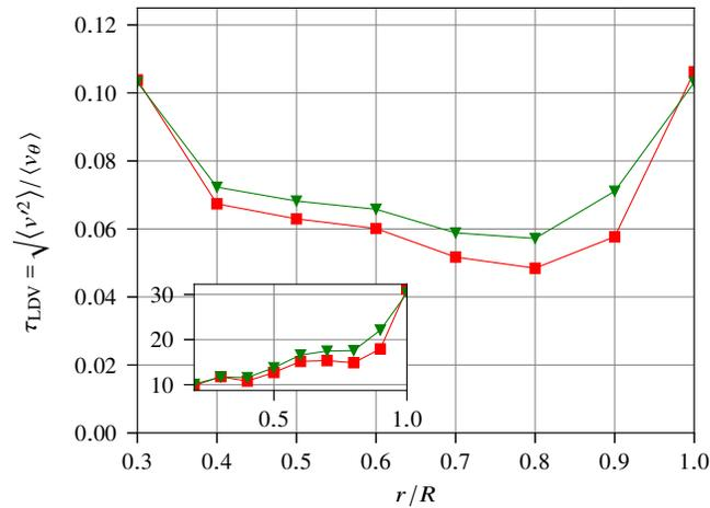
**Figure 5.** Profiles of turbulence intensity, obtained as the ratio of the standard deviation to the mean of the Laser Doppler Velocimetry measurements, at mid-height in the SPHYNX Von Kármán cell. Red squares: azimuthal velocity; green triangles: vertical velocity. The corresponding turbulence intensity close to the wall ( $r/R > 0.8$ ) is between 5% and 10%, both for the azimuthal and the vertical components. Inset: velocity standard deviation in centimeters per second.
