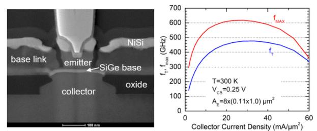
**FIGURE 1.** TEM cross-section of an EEB NSEG SiGe HBT with 110 nm emitter width in 130 nm BiCMOS process (left) and measured  $f_T/f_{MAX}$  vs. collector current density (right).
