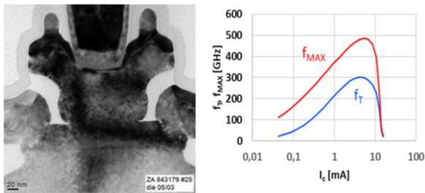
**FIGURE 2.** TEM cross-section of an EBL SEG SiGe HBT in 90 nm BiCMOS flow (left) and measured RF-performance as function of collector current (right). Emitter area is 120 nm x 2.73  $\mu\text{m}$ .
