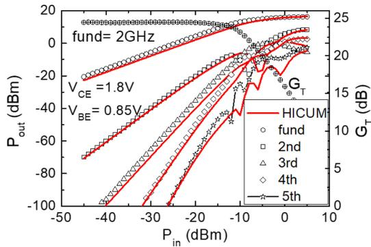
**FIGURE 8.** Output power and all 5 harmonics at fundamental frequency of 2 GHz and  $G_T$  ( $P_{in}$ ) at  $V_{CE} = 1.8$  V. Symbols represent measured data and lines are HICUM. CBEBCx2 CE power cell with emitter area of  $0.13 \mu\text{m} \times 10.16 \mu\text{m} \times 2$ . [30], [31].
