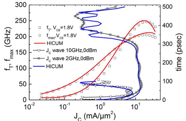
**FIGURE 7.** Current gain cut-off frequency  $f_T$  and maximum oscillation frequency  $f_{MAX}$  at  $V_{CE} = 1.8\text{V}$  and output current density waves at quiescent  $V_{BE} = 0.85\text{V}$  of incident frequency at 2 and 10 GHz.
