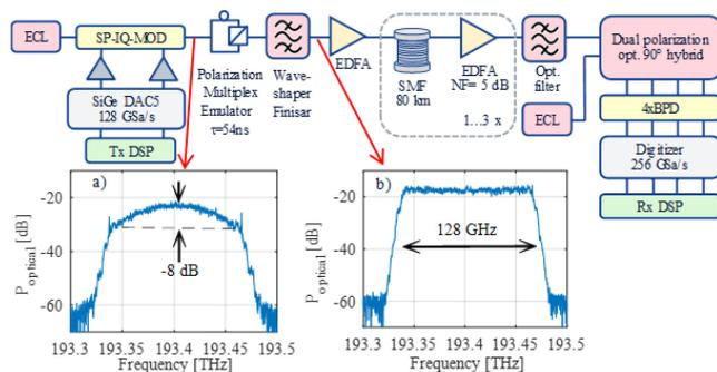
FIGURE 18. Experimental setup of the optical transmission system.
