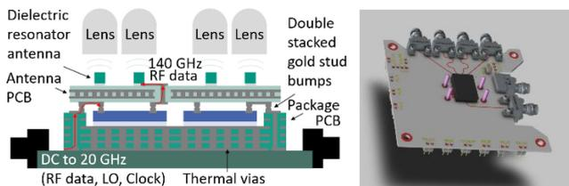
FIGURE 15. Transmitter module stackup (left) and mockup (right).
