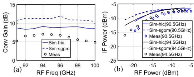
**FIGURE 11.** (a) Conversion gain and (b) IF output power of the mixer as function of RF input power. Comparison between measurement (symbols) and simulation (lines) using two different transistor models.
