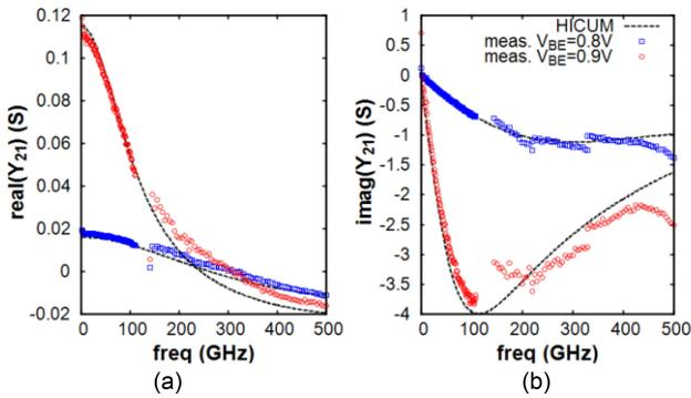
**FIGURE 6.** Comparison between compact model and measurement up to 500 GHz: (a) real part and (b) imaginary part of  $Y_{21}$  versus frequency for  $0.09 \times 4.8 \mu\text{m}^2$  SiGe HBT from STMicroelectronics at  $V_{CB} = 0\text{V}$ .
