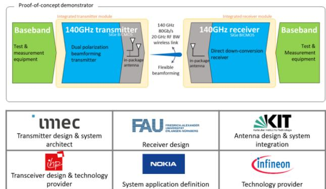
**FIGURE 14. Integrated 6G transceiver system demonstrator.**
