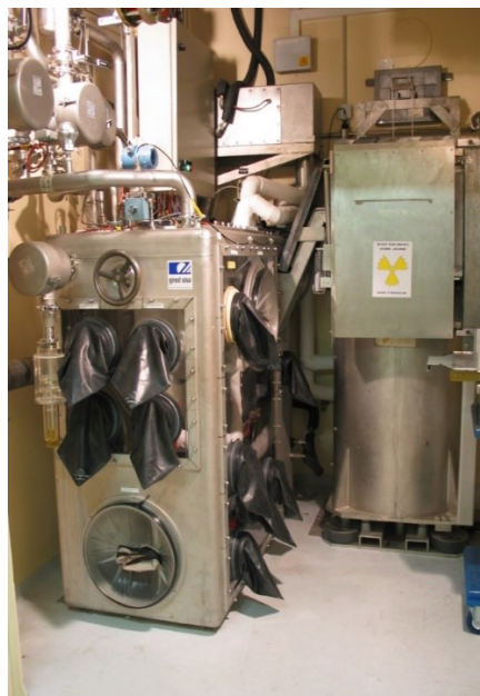
Figure 5 – EPICUR facility to make \gamma -irradiation of ~4L liquid solution
