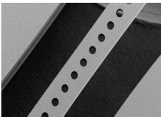
Fig. 5: Microscopic photo of photonic crystal cavity
