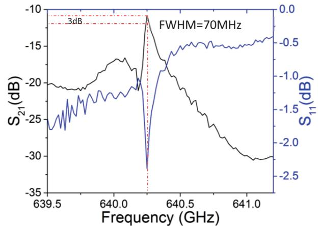
Fig. 7: Measured  $S_{21}$  and  $S_{11}$  of the resonant frequency
