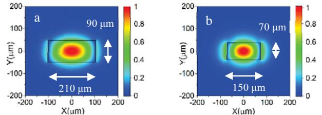
Fig. 1:  $E_x$  of the fundamental mode: (a) multimode structure  $w=210 \mu\text{m}$   $T=90 \mu\text{m}$  and (b) single mode structure  $w=150 \mu\text{m}$   $T=70 \mu\text{m}$
