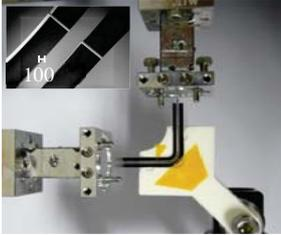
Fig. 3 Suspended Si waveguide on the VNA measurement setup; insert: microscopic image of this waveguide
