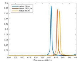
Fig. 6: Resonance frequencies of three different cavities with different etching radius 28, 28.75 and  $29 \mu\text{m}$
