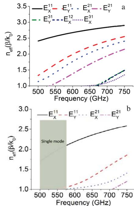
Fig. 2: Propagation constant: (a) multimode structure  $w=210 \mu\text{m}$   $T=90 \mu\text{m}$  and (b) single mode structure  $w=150 \mu\text{m}$   $T=70 \mu\text{m}$
