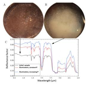
Figure 2: Bidirectional reflectance spectra of the CO<sub>2</sub> slab initial state (black), after thermal cracking (red) and after cracking only due to thermal stress (blue).
