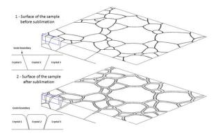
Figure 4: Schematic of the evolution of the sample surface subjected to illumination.
