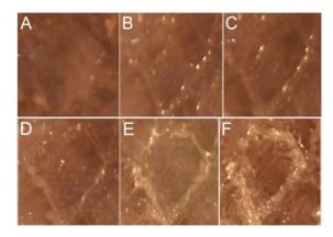
Figure 3: Morphological evolution of CO2 ice grain. During sublimation the grain boundary that separate this grain from the others become brighter.
