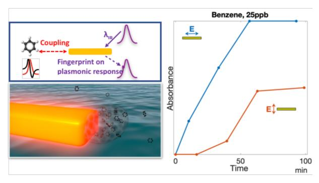
The concerted action of infrared resonant nano-antennas with an ultra-thin zeolite concentrating coating, enables unprecedented rapid detection of benzene traces (25 ppb). In this hybrid material, the zeolite coating effectively traps VOCs analytes nearby the hotspots of nano-antennas, thus enabling Surface Enhanced Infrared Absorption (SEIRA). Sensitivity equivalent to a  $\sim$ 120 m long optical path is achieved in a  $\sim$ 200 nm layer.
