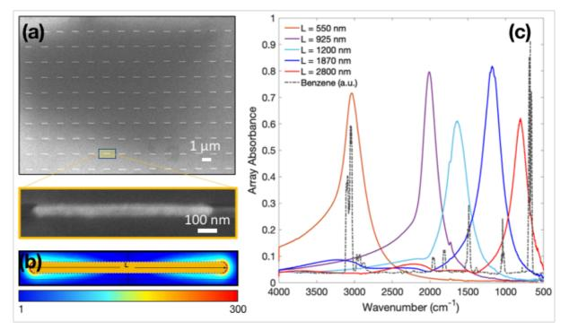
**Figure 3**: (a) SEM image of a resonant nano-antenna array composed of phased gold nanorods. (b) Field distribution at resonance, normalized by the incident field. (c) IR spectra of nanoantenna array of different length overlapped with benzene spectrum (dotted spectrum).
