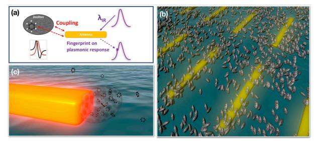
**Figure 1:** (a) Surface-Enhanced Infrared Absorption (SEIRA) concept: near-field coupling between molecular/phonon transitions and optical resonances enables the amplification of the fingerprint. (b) Gold nanorods array coated by zeolite nanocrystals able to trap benzene in regions where the near field enhancement is the highest (c).
