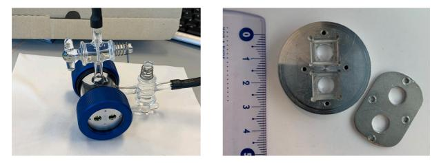
Figure S1. Gas cell featuring a custom metal lid with two orifices where the samples are placed and fixed.
