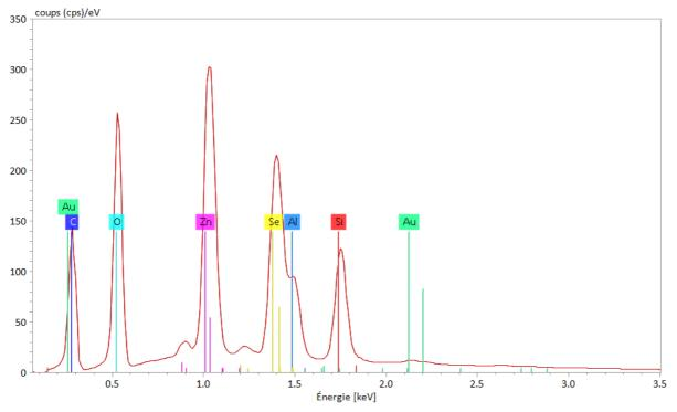
Figure S5: EDX spectrum corresponding to elemental maps shown in Figure 4.
