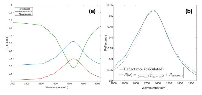
Figure S9: FDTD simulations of the nano-antenna array response (left), FIT of the Reflectance according to temporal coupled mode theory
