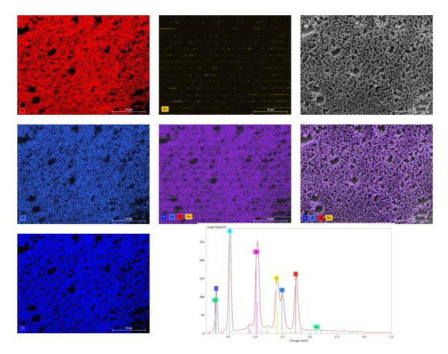
Figure S4: Elemental compositions mapping for a FAU coating on nanoantennas and EDX analysis
