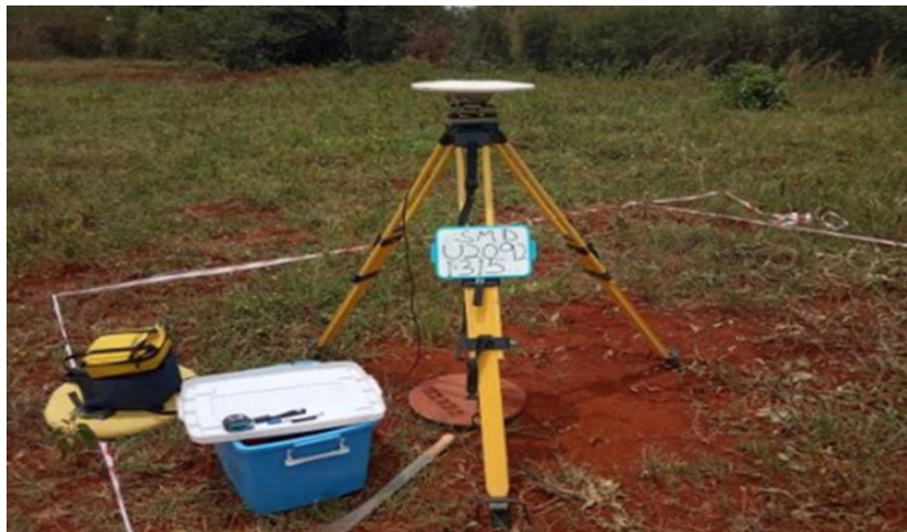
Figure 3 GNSS Receiver at Station U2092
