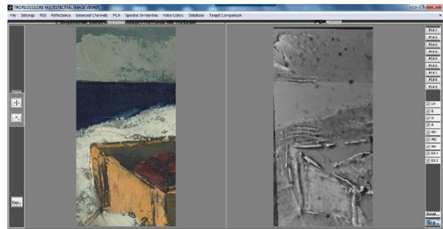
Fig. 1: Screenshot of the image database software, on the left is a photograph of a section of the painting, on the right is a 4<sup>th</sup> principal component fusion of the THz peak to peak transmission amplitude and the x-ray images.
