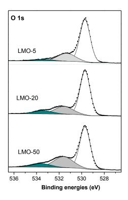
**Figure 5.** O 1s core peaks for the three Li<sub>2</sub>MnO<sub>3</sub> samples with 5%, 20% and 50% of stacking faults before adsorption. The white, grey and green components correspond to the structural oxygen atoms, the surface oxygen atoms and the oxygen atoms of adsorbed species, respectively.
