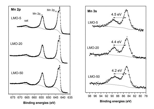
**Figure 4.** Mn 2p (left) and Mn 3s (right) core peaks for Li<sub>2</sub>MnO<sub>3</sub> materials characterized by different contents in stacking faults (S.F.).
