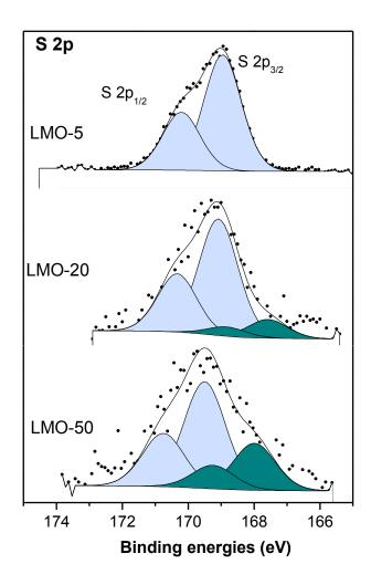
**Figure 6.** S 2p core peaks after adsorption for the three LMO materials.
