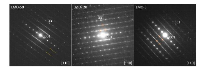
**Figure 2**: Electron diffraction patterns recorded along the [110] zone axis and representative of the compounds LMO-50, LMO-20 and LMO-5. The two yellow arrows on the LMO-50 pattern indicate diffusion lines revealing a high degree of stacking faults. The circles on the LMO-20 and LMO-5 patterns highlight the presence of reflections associated to the monoclinic structure and to the extended ordered structure of Li<sub>2</sub>MnO<sub>3</sub>.
