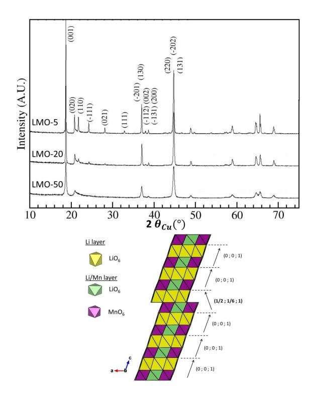
Figure 1. Comparison of the XRD patterns obtained for the three  $\text{Li}_2\text{MnO}_3$  samples with different stacking faults ratios: LMO-SF with SF = 5, 20 and 50, determined by comparison with results reported by Boulineau *et al*<sup>17</sup>(see Figure S2 in supplementary information) (up).
