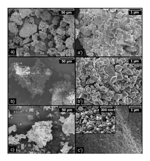
**Figure 3.** SEM images of the three  $\text{Li}_2\text{MnO}_3$  samples: a) and a') LMO-5, b) and b') LMO-20, c) and c') LMO-50.
