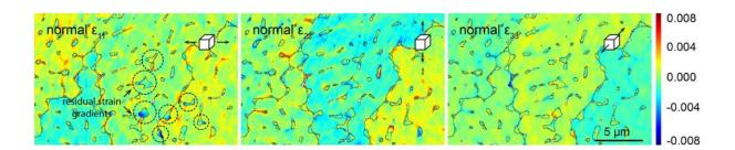
Figure 10 CC-EBSD results of the normal strain components for the Al<sub>0.5</sub>CoCrFeNi sample.
