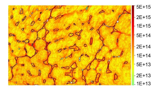
Figure 11 Mapping of GNDs within the microstructure of Al<sub>0.5</sub>CoCrFeNi sample.
