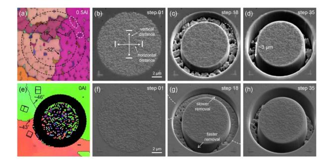
Figure 12 FIB-DIC ring-core milling of HAGBs for (a) to (d) Al<sub>0.5</sub>CoCrFeNi sample and (e) to (h) CoCrFeNi sample. The build directions for both samples are following the out-of-plane directions.
