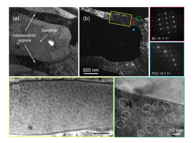
Figure 7. (a) Bright and (b) dark field TEM images of Al<sub>0.5</sub>CoCrFeNi. SAED patterns of dendritic and inter-dendritic regions are coloured in blue and red respectively. (c) Enlarged view of the spinodally decomposed features. (d) HR-TEM of FCC and B2/BCC interface.
