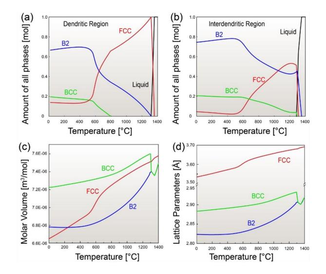
Figure 9 Phase evolution in the (a) dendritic and (b) interdendritic regions of Al<sub>0.5</sub>CoCrFeNi under assumed local equilibrium conditions and using the local compositional enrichment. The molar volumes and lattice parameters of all three phases are plotted in (c) and (d) using the interdendritic compositions, respectively.
