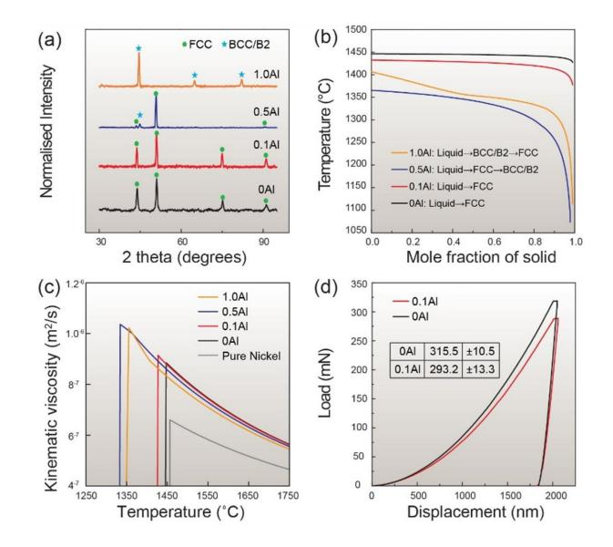
Figure 3. (a) XRD profiles of all samples showing the transition from FCC single-phase regime to BCC/B2 mixture as the AI content increases. (b) Thermo Calc computed solidification paths of all samples under the Scheil condition. (c) Kinematic viscosity values calculated for all samples via the Thermo Calc software. Data for pure Ni was inserted as a reference. (d) Representative nano-indentation curves of CoCrFeNi and Al<sub>0.1</sub>CoCrFeNi.
