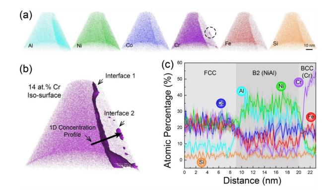
Figure 8. Reconstructed APT volumes for Al<sub>0.5</sub>CoCrFeNi showing (a) elemental distribution, and (b) Iso-surface of 14 at.% Cr. (c) 1D concentration profiles along the line plotted in (b) from FCC phase to B2(NiAI) and finally BCC(Cr) phases.
