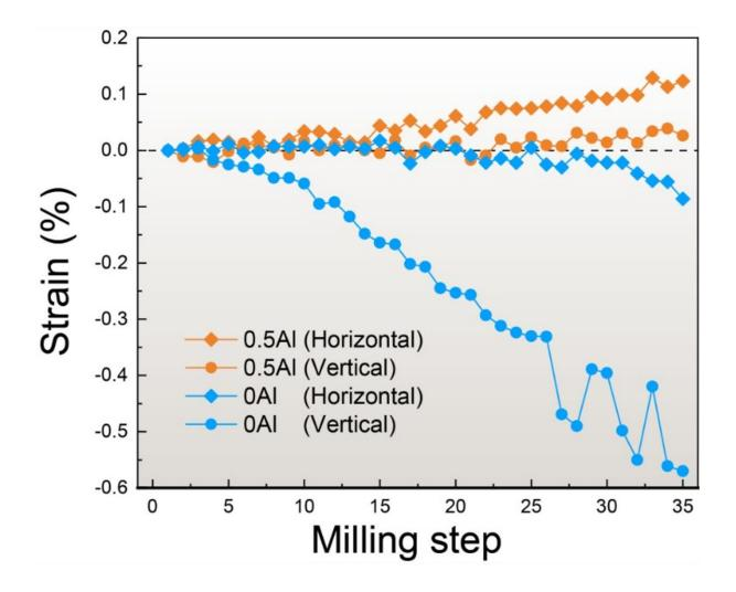
Figure 13 Change in residual strains for the FIB-DIC specimens of 0.5AI and 0AI samples as a function of the milling step (depth).
