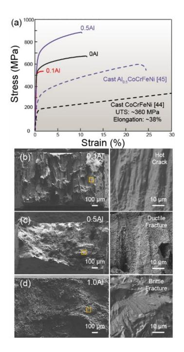
Figure 2. (a) Tensile graphs of SLM-built CoCrFeNi, Al<sub>0.1</sub>CoCrFeNi and Al<sub>1.0</sub>CoCrFeNi with their respective cast counterparts. Representative fracture surfaces of (b) Al<sub>0.1</sub>CoCrFeNi, (c) Al<sub>0.5</sub>CoCrFeNi and (d) Al<sub>1.0</sub>CoCrFeNi.
