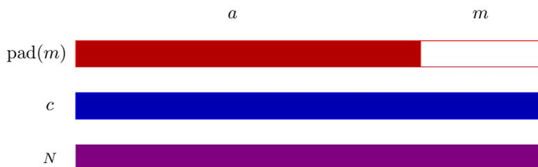
Figure 1: Illustration of low-exponent RSA message recovery attack setup. The attacker knows the public modulus  $N$ , a ciphertext  $c$ , and the padding  $a$  prepended to the unknown message  $m$  before encryption. The attacker wishes to recover  $m$ .
