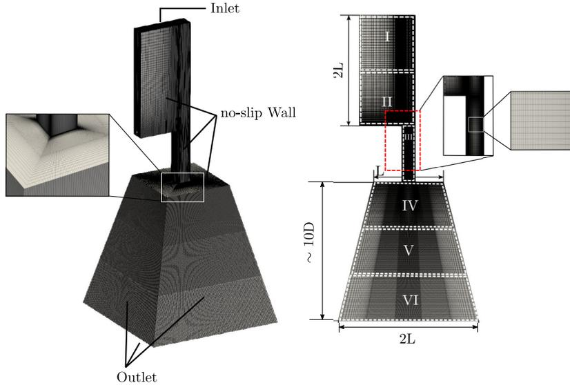
Fig. 20. Injector geometry: domain discretization and refinement regions.
