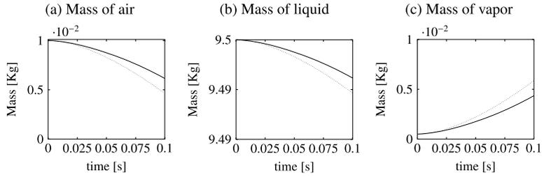
**Fig. 9.** One-dimensional cavitation problem, validation test case. Evolution in time of: (a) air mass; (b) liquid mass; (c) vapor mass. Tests were carried out on two different grids: .... grid A (640 cells); — grid B (1280 cells).
