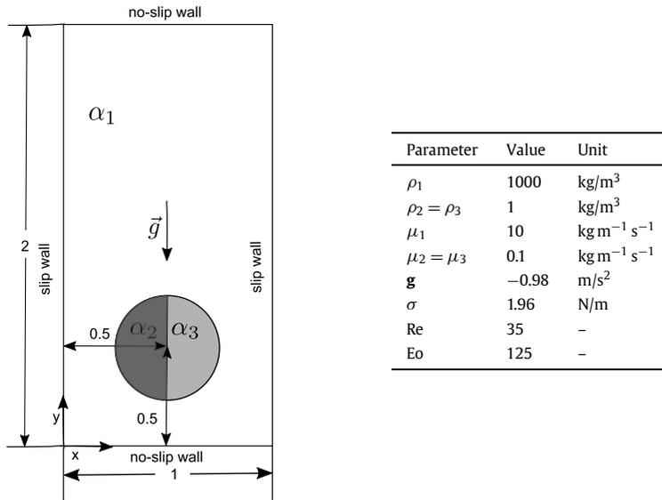
**Fig. 2.** Bubble rising in a liquid column: case setup, boundary and initial conditions. Four different grid resolutions are tested: a)  $40 \times 80$  cells; b)  $80 \times 160$  cells; c)  $160 \times 320$  cells; d)  $320 \times 640$  cells (reference solution).
