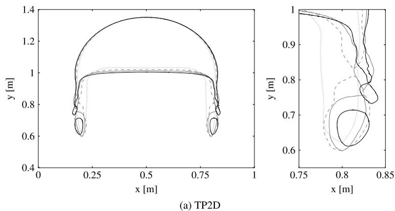
**Fig. 5.** Bubble breakup at time  $t = 3$  s. Comparison of `interPhaseChangeMixingFoam` behavior using four different discretizations: ....  $40 \times 80$  cells; ---  $80 \times 160$  cells; - - -  $160 \times 320$  cells; -  $320 \times 640$  cells.
