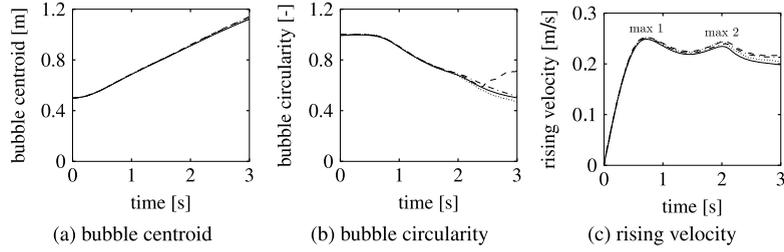
**Fig. 7.** Two-dimensional rising bubble problem, validation test case. Evolution in time of: (a) bubble centroid location  $C$ ; (b) bubble circularity  $C \in [0; 1]$  and (c) bubble rising velocity  $\mathbf{u}_c$ ; circularity is equal to unity if the bubble shape is a perfect circle. Legend: — `interPhaseChangeMixingFoam`, - - - TP2D code, ··· FreeLIFE code, ... MoonNMD [50].
