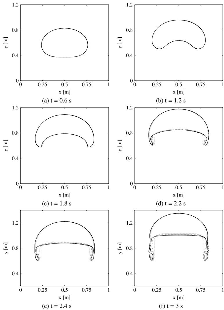
**Fig. 4.** Bubble evolution from 0.6 to 3 s calculated by `interPhaseChangeMixingFoam` on four different grids: ....  $40 \times 80$  cells; ---  $80 \times 160$  cells; - - -  $160 \times 320$  cells; -  $320 \times 640$  cells.
