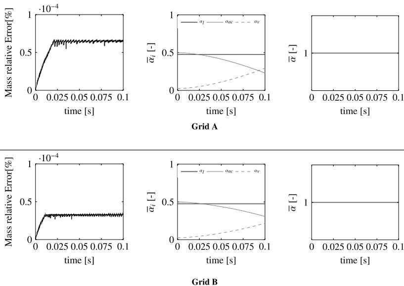
**Fig. 13.** One-dimensional cavitation test case, evolution in time of: left) mass relative error; center) volume-weighted void fractions; right) sum of the volume-weighted void fractions. Grid A:  $1 \times 640$  cells. Grid B:  $1 \times 1280$  cells.
