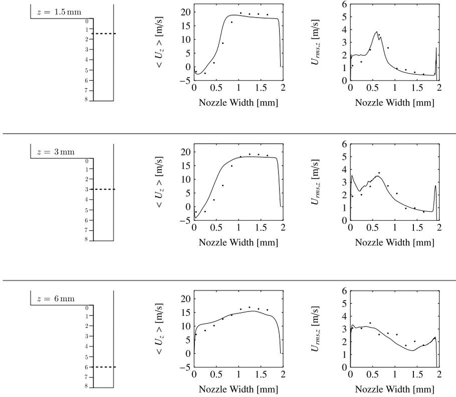
**Fig. 22.** Mean streamwise in-nozzle flow velocity and RMS turbulent velocity at different positions:  $z = 1.55$  mm (top),  $z = 3$  mm (middle),  $z = 6$  mm (bottom); • experiments [52] – `interPhaseChangeMixingFoam`.
