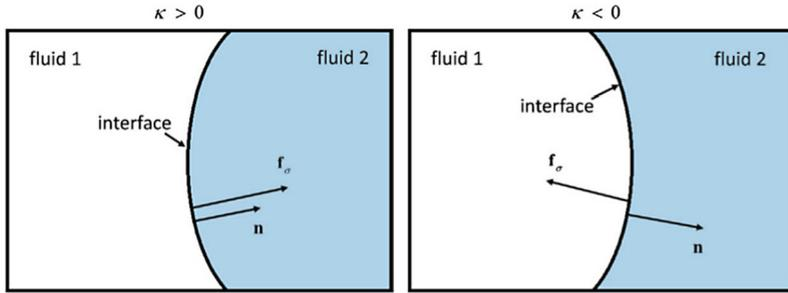
**Fig. 1.** Schematic of the interface between two fluids.  $\mathbf{f}_\sigma$  is the surface force per unit inter-facial area;  $\hat{\mathbf{n}}$  and  $\kappa$  are namely the interface normal and the interface curvature. According to the sign convention adopted,  $\mathbf{f}_\sigma$  is always oriented towards the concave interface and  $\hat{\mathbf{n}}$  always points towards lighter couple of fluids [76].
