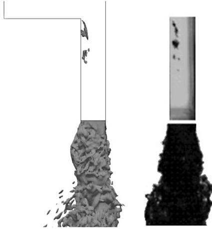
Fig. 21. Internal nozzle flow test case [52]. Left) `interPhaseChangeMixingFoam`; right) visualizations from experiments.
