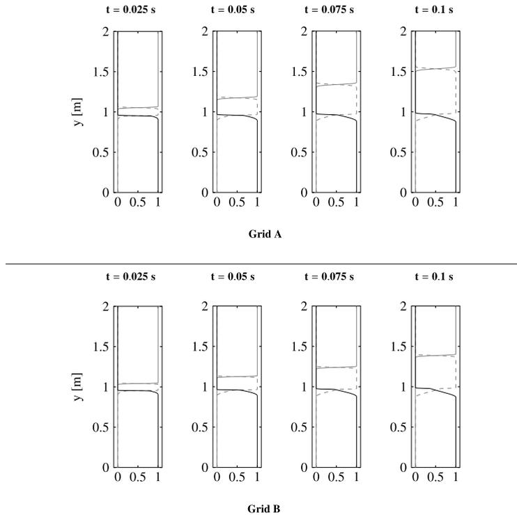
**Fig. 11.** One-dimensional cavitation problem. Evolution of the void fractions from 0.025 to 0.1 s. Top) grid A,  $1 \times 640$  cells; bottom) grid B,  $1 \times 1280$  cells. Legend:  $\alpha_l$  —,  $\alpha_{nc}$  ---,  $\alpha_v$  ....
