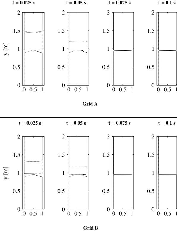
**Fig. 16.** One-dimensional condensation problem. Evolution of the void fractions from 0.025 to 0.1 s. Top) grid A,  $1 \times 640$  cells; bottom) grid B,  $1 \times 1280$  cells. Legend:  $\alpha_l$  —,  $\alpha_{nc}$  ---,  $\alpha_v$  ····.
