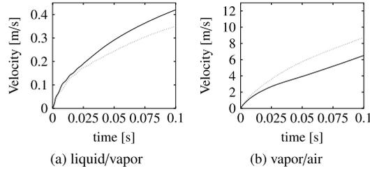
**Fig. 12.** One-dimensional cavitation problem, validation test case. Evolution in time of the mean interface velocity (Eq. (53)): (a) liquid/vapor; (b) vapor/non-condensable gas for two different grids: .... 640 cells; — 1280 cells.
