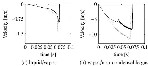
**Fig. 17.** One-dimensional condensation problem, validation test case. Evolution in time of the mean interface velocity (Eq. (53)): (a) liquid/vapor; (b) vapor/non-condensable gas for two different grids: ···· 640 cells; — 1280 cells.
