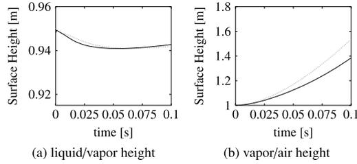
**Fig. 10.** One-dimensional cavitation problem, validation test case. Evolution in time of the surface heights: (a) liquid/vapor, (b) air/vapor on two different grids: .... grid A (640 cells); — grid B (1280 cells).
