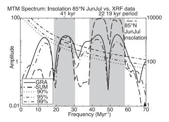
**Figure 7.** Interval "c" in Figure 1, modified from *Sangiorgi et al.* [2008b]. Multitaper spectral analysis of insolation, GRA bulk density, and summary signal extracted by MSSA from combined bulk density, magnetic susceptibility, XRF-derived Ti, Al, and K, and natural gamma measurements.
