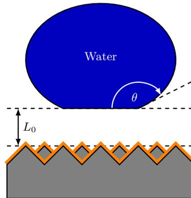
FIG. 1. (Color online). Sketch of the studied system. At equilibrium, the water droplet is separated from the nanostructured surface by the distance  $L_0$ <sup>16</sup>. The droplet presents a contact angle  $\theta$ . The nanostructured silicon (grey) is coated (orange) with organic molecules in order to emulate a nanostructured molecular solid surface.
