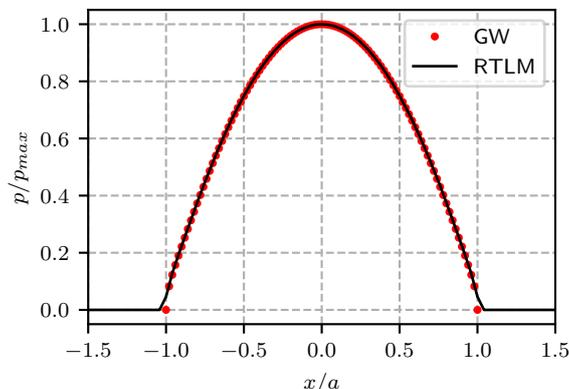
Figure 13: Comparison of the resulting pressure distribution for Greenwood solution (GW) and RTLM contact simulation implemented in ABAQUS. (Indenter of shape  $\phi = x^2/2R$ , where  $R = 50$  and  $a/e = 5$ .)
