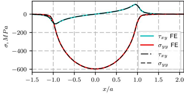
(b) Stress along  $\Gamma(\hat{y} = 0)$  (coating substrate interface)
