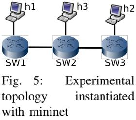
Fig. 5: Experimental topology instantiated with mininet
