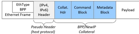
Fig. 1: BPP Packet Structure
