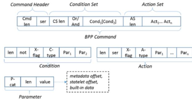
Fig. 3: BPP Command Structure
