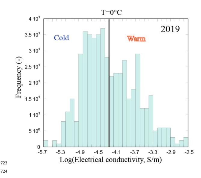
Figure 8. Distribution of the electrical conductivity for the 2019 field data. We observe a
