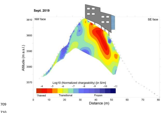
Figure 6. Normalized chargeability tomograms (in S m<sup>-1</sup>) of the rock ridge below the Cosmiques refuge in 2019. Tomogram is smaller in SE face due to the lack of inverted data points.
