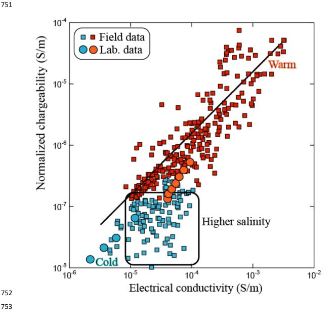
Figure 11. Normalized chargeability versus electrical conductivity. Comparison between the field and laboratory data (PAS1). The color code is blue for the cold values below the freezing temperature and red above the freezing temperature. The plain line corresponds to the best fit of the field data (with a slope of 0.016, r = 0.69). The small value of the slope (smaller than R = 0.10 indicates that conductivity is mostly dominated by the pore water contribution.
