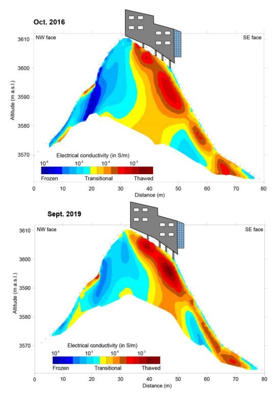
**Figure 5.** Electrical conductivity tomography (in S m<sup>-1</sup>) of the rock ridge below the Cosmiques refuge in 2016 and 2019. We use cold colors for the low conductivity values presumed to correspond to the rock mass undergoing freezing conditions. The warm colors corresponds to the rock mass above freezing conditions.
