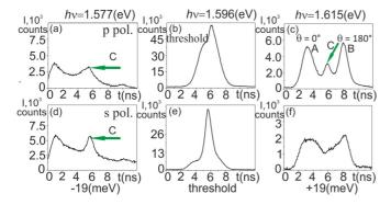
FIG. 3. Time-of-flight spectra taken at three photon energies close to the photoionization threshold with a wide bandwidth of the Ti:sapphire laser ( $\Delta E = 24 \,\mathrm{meV}$ ). (a)–(c) with *p*-polarized light; (d)–(f) same but for *s*-polarized light.
