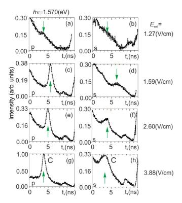
FIG. 4. Dependence of the field-ionization spectra on the strength of the extraction field. Measurements were performed with ionization-laser bandwidth  $\Delta E = 24 \,\text{meV}$ , energy below threshold  $-19 \,\text{meV}$ . (a),(c),(e),(g) *p*-polarized light, (b),(d),(f),(h) *s*-polarized light.
