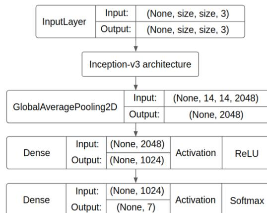
441 **Fig. 12:** Developed architecture based on InceptionV3.
