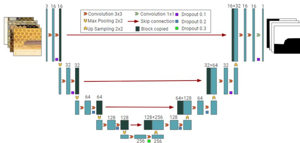
336 **Fig. 7:** CNN architecture based on U-Net to handle comb segmentation.
