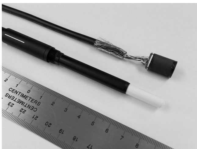
Fig. 12. A prototype of the Graphite Probe Calorimeter without its waterproof housing, next to a Sun Nuclear SNC 600c Farmer chamber for scale. The cylindrical graphite core (not visible) has a length of 10 mm and a diameter of 6.1 mm.
