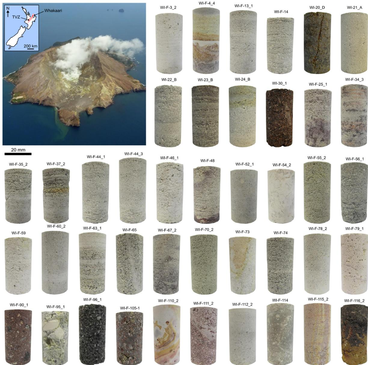
**Fig. 3.** Photographs of the experimental samples (20 mm in diameter and nominally 40 mm in length) from Whakaari (New Zealand) (photographs of duplicate cores, cored from the same block, are omitted). Top left shows a photograph of Whakaari; inset shows a map of New Zealand with the locations of the Taupō Volcanic Zone (TVZ) and Whakaari indicated.
