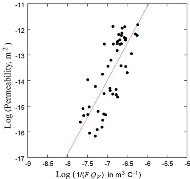
**Fig. 7.** Permeability as a function of alteration indicator (see text for details) for the rock samples from Whakaari (New Zealand). The solid line corresponds to the fit discussed in the main text. The coefficient of correlation is  $R^2 = 0.60$ . The fitted parameters are discussed in the main text.
