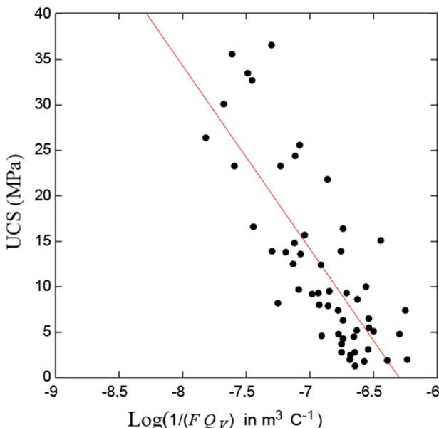
**Fig. 8.** Uniaxial compressive strength (UCS) as a function of alteration indicator (see text for details) for the rock samples from Whakaari (New Zealand). The solid line corresponds to the fit discussed in the main text. The coefficient of correlation is  $R^2 = 0.61$ . The fitted parameters are discussed in the main text.
