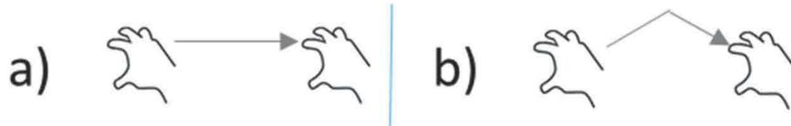
**Fig. 1.** Tolerance of *swipe* touch interaction techniques to hardware faults (loss of a line in the hardware grid) – (a) non tolerant (b) tolerant
