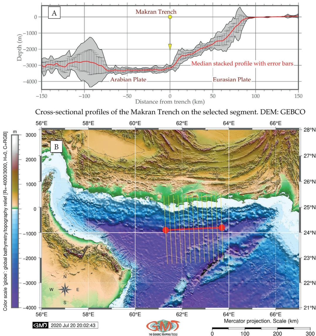
Fig. 6. Makran Trench: cross-section profiles and graph
