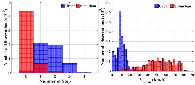
Fig. 6(a). Histogram on  $NoS$  and  $v_{\text{mean}}$  of driving samples (per 75s) under urban and suburban patterns.
