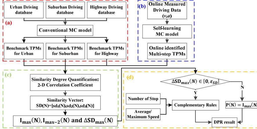
Fig. 3. Working flow of the proposed MC driving pattern recognition approach.
