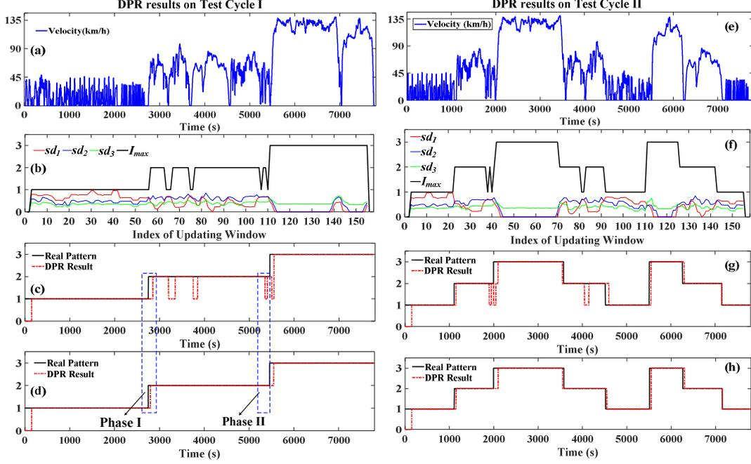
Fig. 8 (a)-(h). DPR results on test cycle I, II. Fig (a) and (e): Multi-pattern speed profile. Fig (b) and (f): Similarity quantification results. Fig (c) and (g): DPR results without complementary rules. Fig (d) and (h): DPR results with complementary rules.
