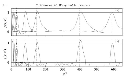
FIGURE 2. Shape of the correlation function calculated from the DNS database at 7 different y-locations:  $y^+ = 4$ ;  $y^+ = 14$ ;  $y^+ = 30$ ;  $y^+ = 80$ ;  $y^+ = 150$ ;  $y^+ = 400$ ;  $y^+ = 590$ . Separations in the x- and z-directions are zero. f(x, x') is evaluated from (4.5) with: (a)  $\alpha = \beta = 1$ ; (b)  $\alpha = \beta = 2$ . For clarity, curves have been truncated at large separations.
