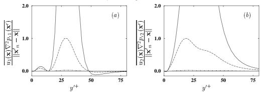
FIGURE 1. Comparison of the three terms in the integrand of (4.3) at  $y^+ = 30$  for separations in y-direction. (a) Integrand of  $\phi_{11}^*$ ; (b) Integrand of  $\phi_{22}^*$ . — principal term (n=0); — image term due to the wall at  $y^+ = 0$  (n = -1); —— image term due to the wall at  $y^+ = 1180$ (n = 1). The vertical coordinate is arbitrarily normalized such that the maximum of n = -1term is 1.
