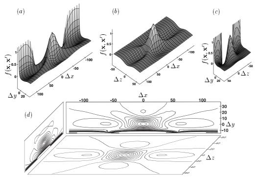
FIGURE 6. Shape of the correlation function defined by (4.5) with  $\alpha = \beta = 1$  at  $y^+ = 14$ . (a) Separation in x-y plane; (b) Separation in x-z plane; (c) Separation in y-z plane; (d) Iso-correlation contours in these three planes (21 contours from 1 to -1 are plotted).
