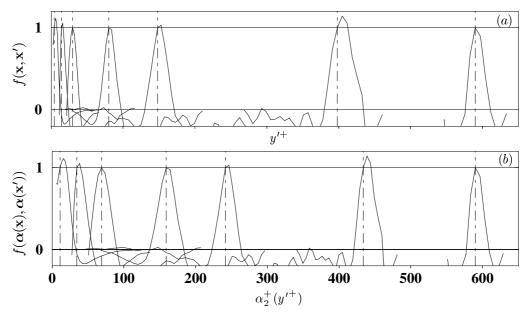
FIGURE 14. Effect of the space transformation on the correlation function: (a) Correlation function in the original space  $\Omega$  (same as figure 2b); (b) Correlation function after transformation of  $y^+$ -axis. See figure 2 for additional caption.
