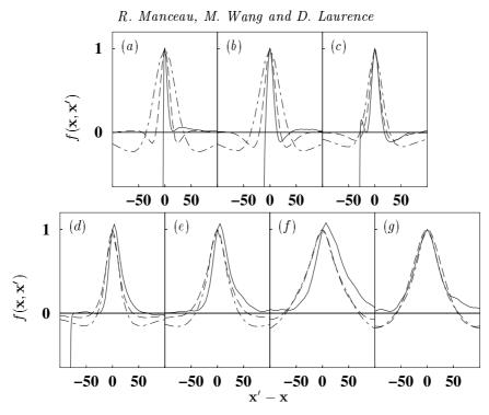
FIGURE 4. Shape of the correlation function defined by (4.5) with  $\alpha = \beta = 1$ , evaluated from the DNS data, in the 3 principal directions, at 7 different y-locations. (a)  $y^+ = 4$ ; (b)  $y^+ = 14$ ; (c)  $y^+ = 30$ ; (d)  $y^+ = 80$ ; (e)  $y^+ = 150$ ; (f)  $y^+ = 400$ ; (g)  $y^+ = 590$ . Separations: ---- x-direction  $(\Delta y = \Delta z = 0)$ ; ---- y-direction  $(\Delta x = \Delta z = 0)$ ; ---- z-direction  $(\Delta x = \Delta y = 0)$ .
