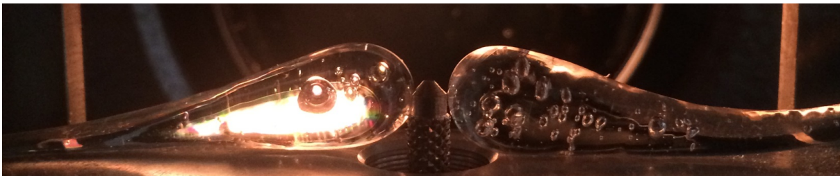
Figure 8: Picture of two glass drops observed under polarized and analyzed light. The sample at the left is unrelaxed, while that at the right was annealed, removing any intern stress. Picture courtesy of Prof. D. de Ligny.
