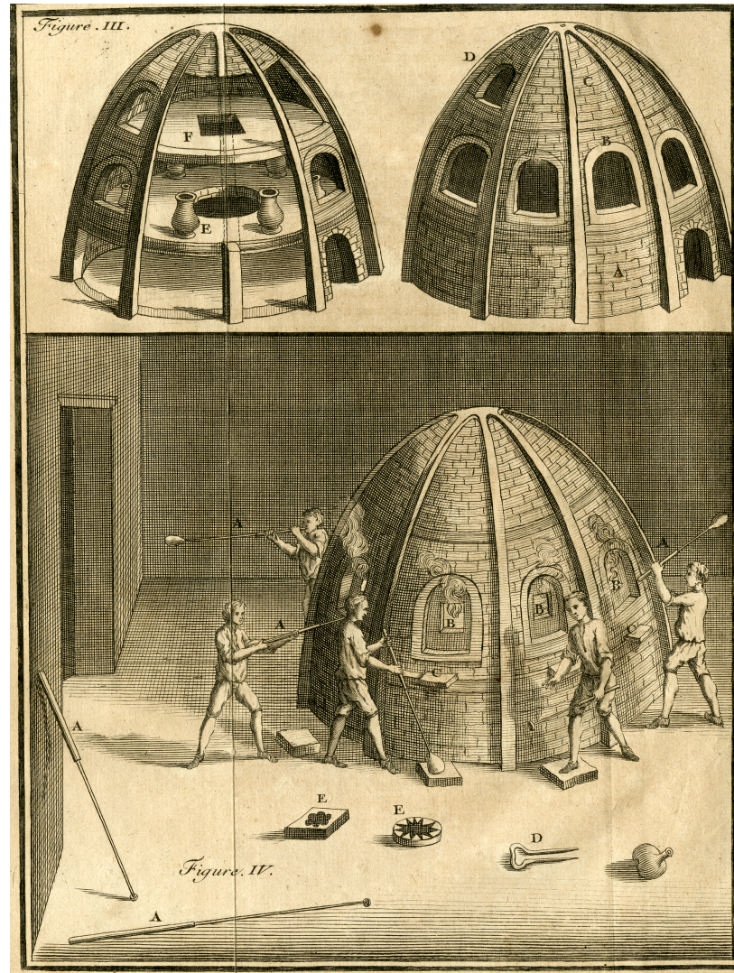
Figure 7: Representation of the three different furnaces needed to make glass and proposed by Agricola. This representation is extracted from “Dans l’art de la verrerie” from Neri, Merret and Kunckel (1752) [6].
