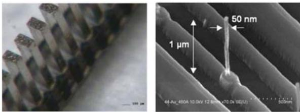
**Fig. 4.** Example of a THz slow wave structure realized using LIGA technique (20 to 200  $\mu\text{m}$  typ. period with an aspect ratio  $> 1:10$ ) (left). Example of a CNT grown on a "diffractive" structure. It provides an alignment of the polarization of the modulated optical beam (i.e. of the corresponding electric field) onto the main dimension of the CNTs (right).
