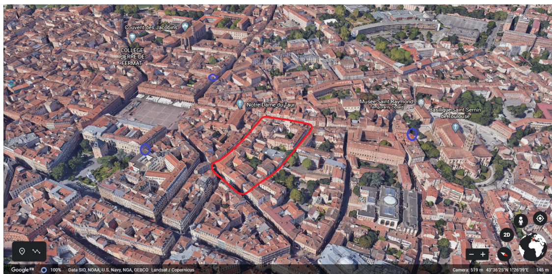
Figure 4. 3D Image of the Urban Scenario with the mobile agent's real trajectory (red), and the three LTE antennas (blue circles).
