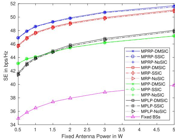
**FIGURE 5. Spectral efficiency of the different UAV positioning techniques and PA strategies.**
