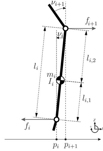
Figure 12: One segment  $s_i$  of the model.
