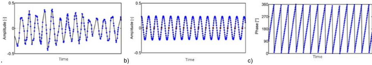
**Figure 3.** Profile of pressure signal. a) initial signal. b) filtered signal. c) zero crossings according to acquisition time. Length of a period is around  $\frac{1}{33}$  s.
