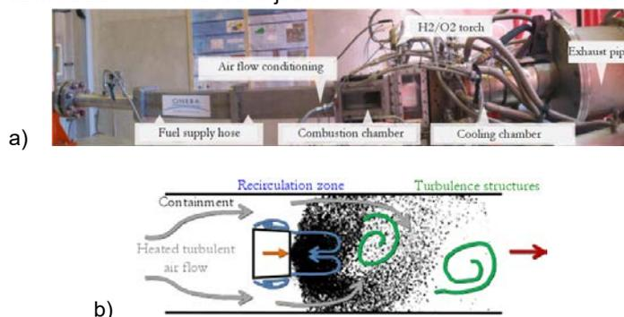
Figure 1. a) View of the experimental test rig. b) Sketch of the combustion chamber
