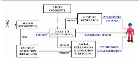
Fig. 1: Overview of the system architecture
