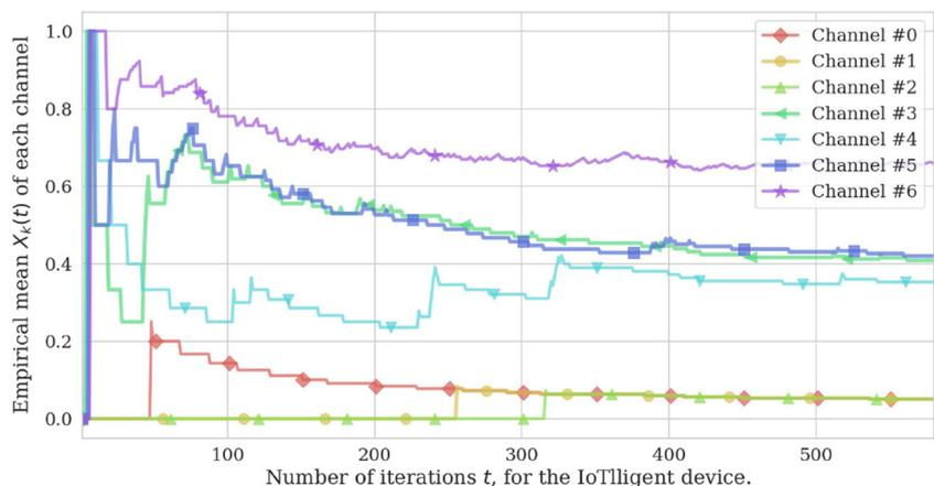
**Fig. 17** Evolution of the  $X_k$  empirical mean through time of reference IoT device for scenario 2
