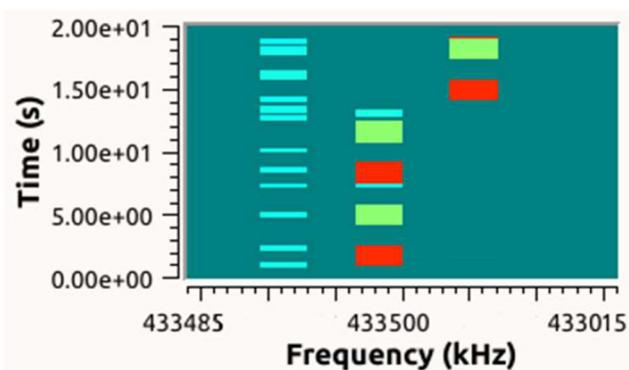
**Fig. 3** Spectrum waterfall view on GRC received at gateway side in a 4 channels example (only 3 occupied in this picture), during experiments. Time is in y-axis (going down) and frequency in x-axis. Blue short transmissions are those produced by the traffic generator, green blocks are our IoT transmissions, and red blocks are the gateway transmissions itself
