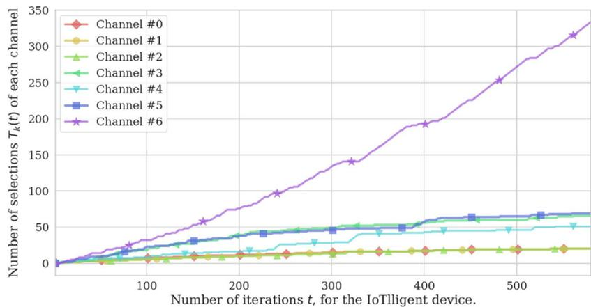
the use of less occupied channels and especially channel #6 which is completely vacant.
