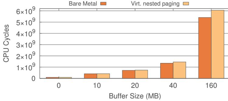
Fig. 9. Median enclave startup time (lower is better)
