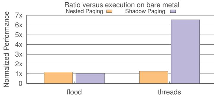
Fig. 14. Normalized benchmark run time (lower is better)
