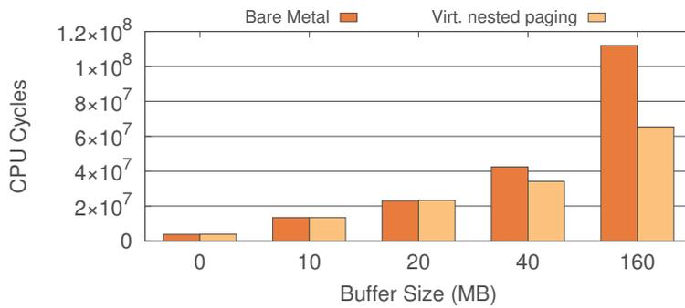
Fig. 10. Median enclave shutdown time (lower is better)
