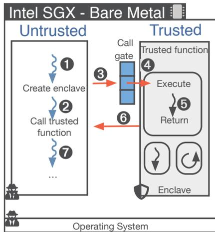
Fig. 1. Intel SGX workflow on bare metal environments.
