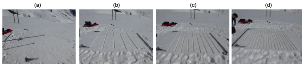
Figure 2. Studied surfaces of experiment A (Table 1), from (a) to (d): A smooth, A \eta 7\% , A \eta 13\% and A \eta 27\% sites.
