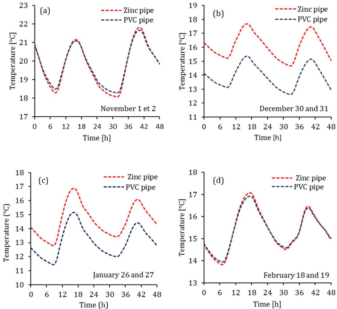
485 Fig. 21. Viewing the effect of the pipe material on air temperatures at the outlet of two
