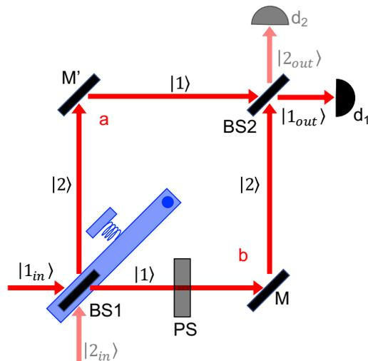
FIG. 4. Scheme of the Mach-Zehnder interferometer with a movable beam splitter BS1, a phase shifter with  $\phi$  with two possible incoming beams  $|1_{in}\rangle$  and  $|2_{in}\rangle$  and outputs  $|1_{out}\rangle$  and  $|2_{out}\rangle$  measured by the detectors  $d_1$  and  $d_2$ . Photons parallel to the incoming photon (horizontal propagation in the figure) are indicated by the states  $|1\rangle$  and with  $|2\rangle$  otherwise (vertical propagation).
