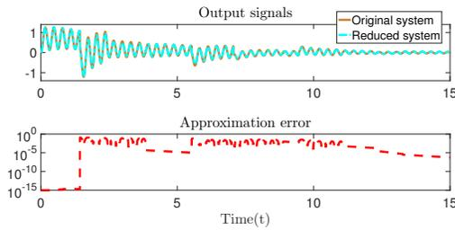
Fig. 4. The observed outputs for the original and reduced systems and the deviation between them (for the first choice of  $r_k$ 's).
