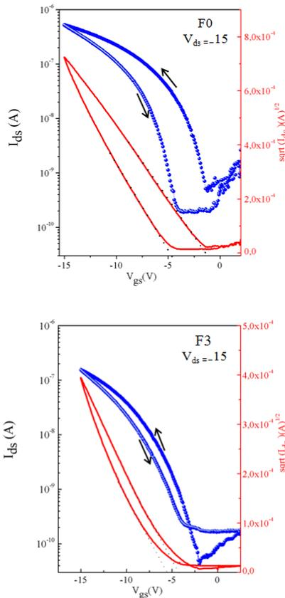
**Figure 1.** a) Bottom gate, top-contact field-effect transistor device used in this work, b) transfer characteristics of the OFET devices in saturation regime with **F0** and **F3** as the active layer. Threshold voltage was determined by extrapolating  $\sqrt{I_{ds}}$  to zero current. Hysteresis was quantified by the difference in the threshold voltages ( $\Delta V_{th}$ ) of forward and backward scan as shown in the figure as dashed lines.
