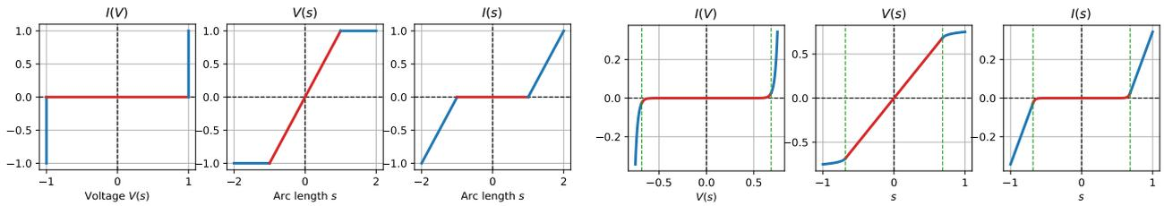
Figure 4: (Pseudo) Arc-length parametrization of hard clipping resistor and anti-parallel Shockley diodes.
