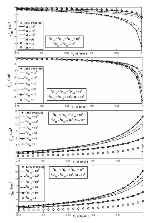
Fig. 3 Effect of the mechanical/electrical imperfection parameters on the effective piezoelectric coefficients  $e_{311}^*$ ,  $e_{113}^*$  and  $e_{223}^*$  for a bilaminate composite PZT-5A/Araldite
