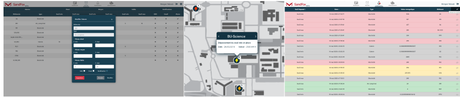
Fig. 2. left, Dialog box for creating an alarm; centre, display of notifications on the Map; right, interface listing the information of each detected anomaly
