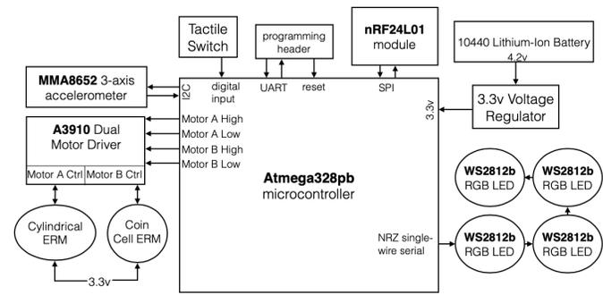
Figure 2: A system overview showing the hardware configuration of a single Vibropixel.
