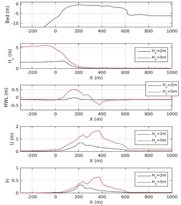
Figure 3. Comparison between two numerical cases performed by the wave-resolving SWASH model:  $H_s=2$  m,  $T_p=12$  s and  $H_s=5$  m,  $T_p=16$  s, in black and red lines, respectively. From top to bottom, the 20-min averaged cross-reef distribution of: reef bathymetry, significant wave height, depth-averaged velocity and Froude number.
