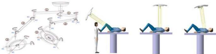
**Fig. 1.** (left) Kinematics of standard lighting arm for operating room; (right) typical positions of the lighting dome in an operating scene
