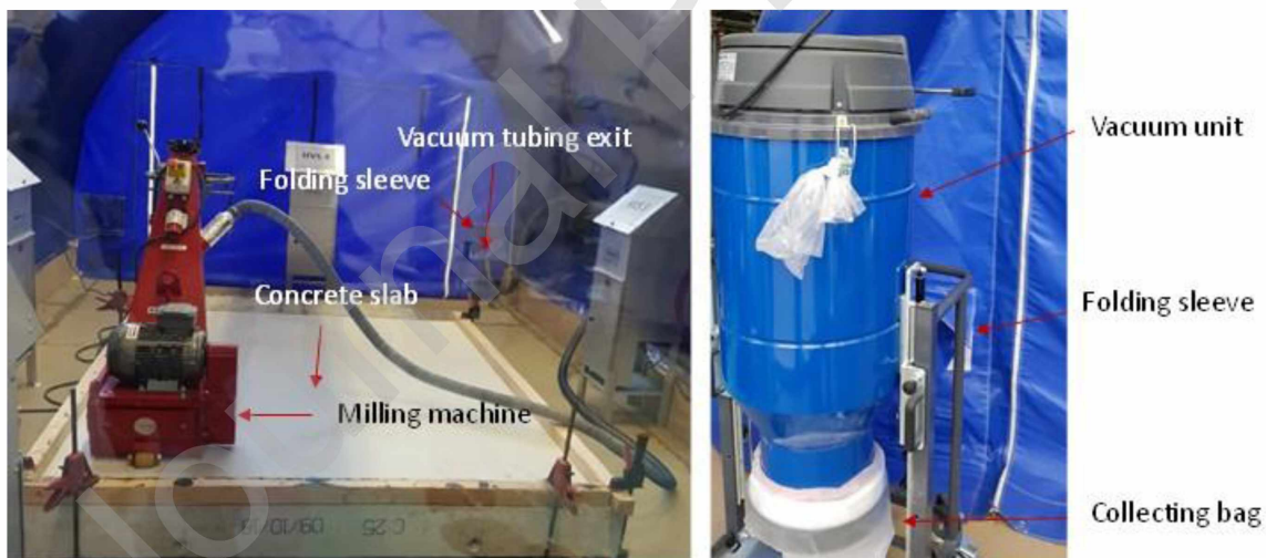
Figure 1 - The Blastrac milling machine equipped with a tubing sitting on the concrete slab (left) and the vacuum dust collector with its bagging system
