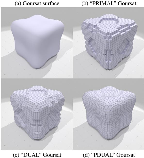
**Figure 4:** Possible input shapes for convergence tests, given input polynomial Goursat surface  $3(x^4 + y^4 + z^4) - 200(x^2 + y^2 + z^2) = 800$  digitized at gridstep  $h = 1$ : (a) continuous polynomial surface, (b) digital surface bordering interior voxels, (c) dual surface to “PRIMAL” surface, (d) projection of “DUAL” vertices onto continuous surface.
