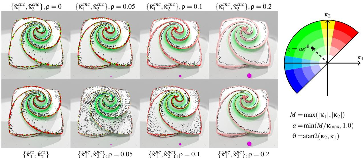
**Figure 13:** Extraction of convex (red), concave (blue), hyperbolic (green), concave/convex cylindrical (cyan/yellow) and flat parts (white) on “Octaflower” dataset. Colors are computed as explained by the right diagram, with  $\kappa_{\max} = 4$ , and  $\kappa_1 \leq \kappa_2$ .
