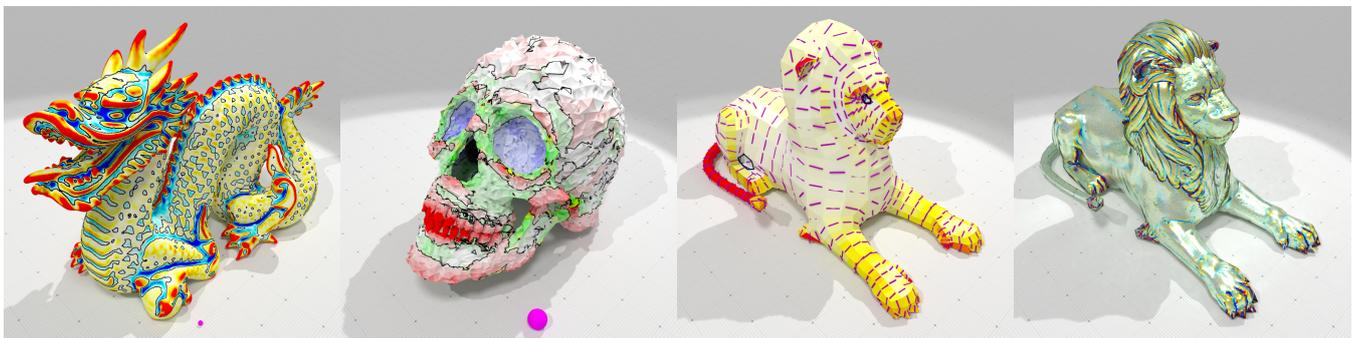
**Figure 1:** Left: mean curvature estimation. Middle left: convex, concave and saddle parts estimation on noisy data. Middle right: second principal curvature and direction estimation on coarse “Lion” mesh. Right: mean curvature extraction on the same “Lion” mesh geometry but with normal vector field given by normal map.
