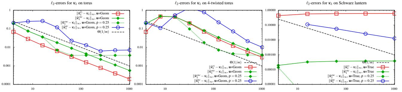
**Figure 5:** Pointwise convergence for first principal curvature: in abscissa, parameter  $m$  giving the number of transversal slices, in ordinate  $\ell_2$ -error estimation of first principal curvature. **Left:** torus with  $n = m$ . **Middle:** 4-twisted torus with  $n = m$ . **Right:** Schwarz lantern with  $n = \sqrt{m}$ .
